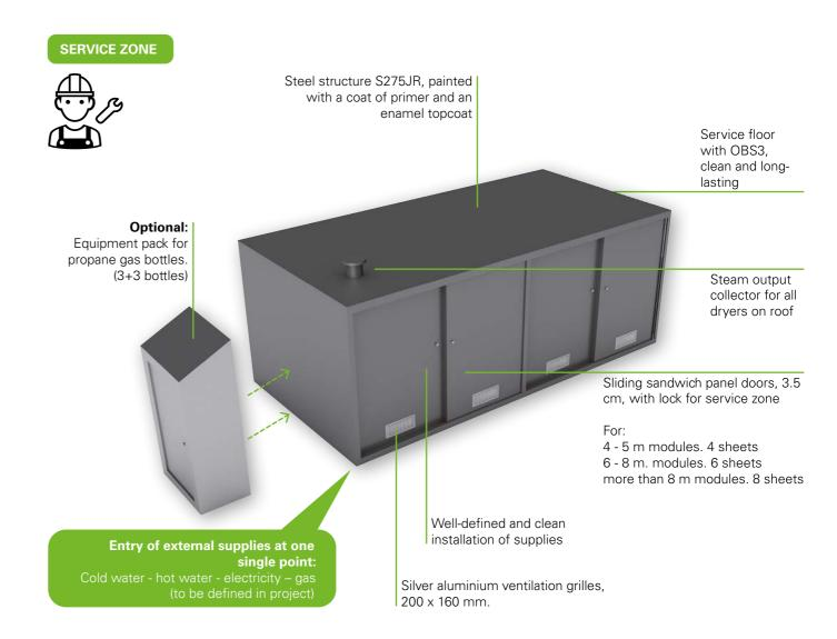
The module is designed for transportation with the machines inside.
