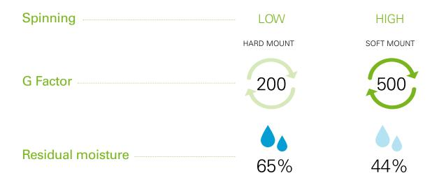
This translates directly in more efficiency in the drying cycle, with a high spin washer, as the drying cycle is much shorter.
