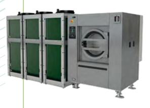
In a DHS-80C TOUCH II washer we can achieve up to 56% water savings thanks to ECOTANK XL if we load 60% of the capacity, with towels.
